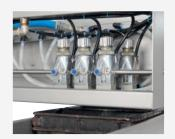
B Customized solutions: Different positions of the spray guns are possible (e.g. 6 in a row, 2 rows of 3)
