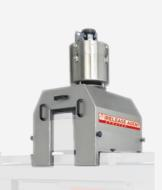
Exhaust unit with microfilter An exhaust unit can be placed over the spray hood to suck up excessive oil mist that is created during spraying. Centrifugal force will separate the oil from the air. The removed oil is discharged via a hose and collected in a container. Clean air is blown out through the filter.
