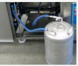
This container is constantly under pressure to feed the spray guns.
